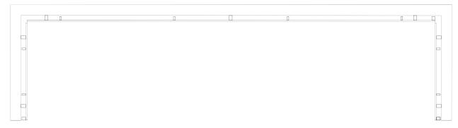
When measuring, first of all take the measurements directly into the corners of the bay for both the front and the side blinds. For the width of the blind for the front, reduce the corner to corner measurement by 90mm, this will allow for the 45mm space that is required either side. For the widths of the side blinds, reduce the corner to corner measurement by 45mm. Finally, order all three of your blinds as 'exact fitting'.
