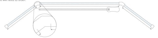
To establish your drop, measure from where the top of the blind will sit, down to where you want the blind to stop (normally the windowsill). With the measurements for the widths and the drops of your blinds, all you need to do now is enter them into our site, and order them with an 'Exact' measurement type and the 'Bracket to Bracket' option selected.
